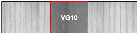
Under microscope at 100x magnification The VG10 core material is clad by 18 layers on each side (=37 total)
